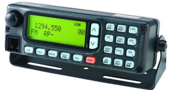
Control head for Icom ID-1 1.2 GHz D-STAR digital transceiver
