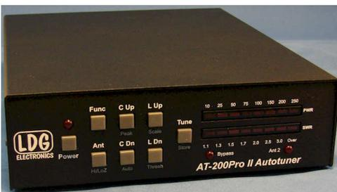
The LDG Electronics AT-200ProII automatic antenna tuner handles up to 200 watts SSB or CW on 1.8 to 30 MHz, and 100 watts on 54 MHz. Its processor-controlled switched-L tuner matches any coax-fed antenna, including yagis, dipoles, inverted V's, slopers, loops, etc. It typically matches a 10:1 SWR down to 1.5:1 in a few seconds. It can also be used with long wires, random wires, and antennas fed with ladder line, with an optional balun.
