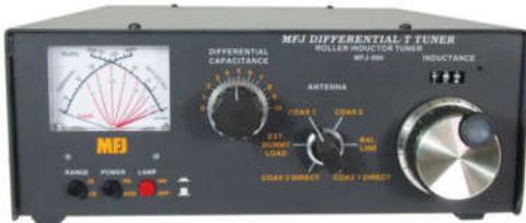
The MFJ-986 differential-T antenna tuner uses ganged differential capacitors (one increases capacitance while the other decreases) and a roller inductor for fast two-knob tuning. It handles 1.5 kW output power over 1.8 to 30 MHz. Its six-position antenna switch selects two coax lines and/or random wires (direct or through the tuner), balanced line, and internal dummy load.
