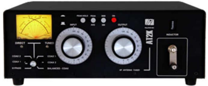
The Palstar AT2K antenna tuner covers 160 to 6 meters with a power rating of 2000 watts PEP. A small roller inductor allows tuning on 6 meters, and 400-pF maximum capacitance provides low-band performance. It matches dipoles, center-fed doublets, verticals, end-fed wire, delta loops, beams, Windoms, and inverted V's. Included is a six-position antenna selector switch. An external 4:1 current
