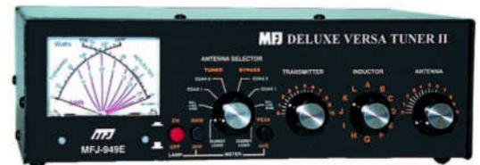
The MFJ-949E 300-watt antenna tuner covers 1.8 to 30 MHz. It includes a tapped inductor with switch and two variable capacitors, and tunes out SWR on dipoles, verticals, inverted V's, random wires, beams, etc., fed with coax, random wire, or balanced lines. It also includes a 4:1 balun. A three-position antenna switch selects two coax-fed antennas, random wire/balanced line, or built-in dummy load through the tuner or direct to the radio.
